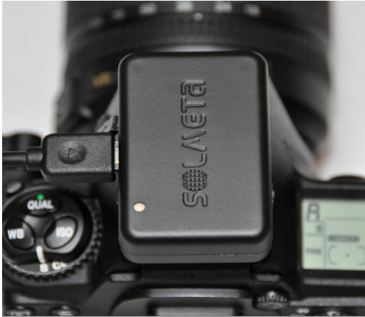
Slide the unit onto the hot shoe
