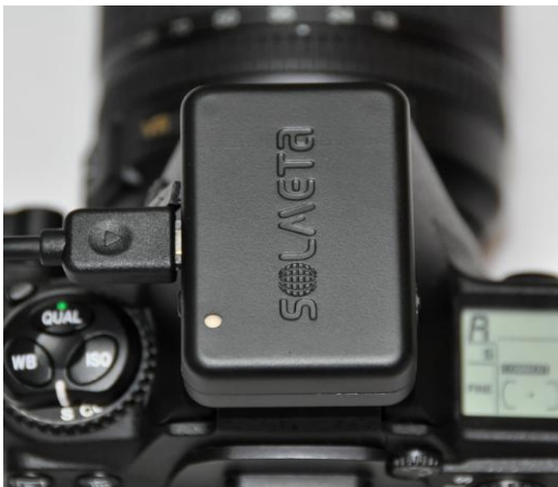
Slide the N1 onto the hot shoe
